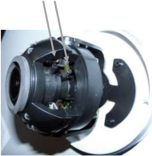
Picture 4: Lens adjustment (zoom and focus):
